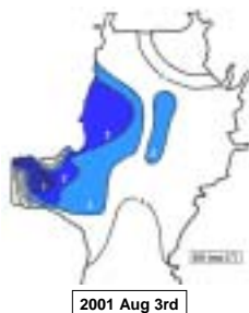
DO distribution at the bottom of Ariake Sea (by Tsutsumi et al. 2003)
