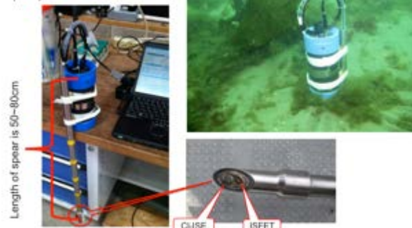
Spear pH/ORP sensor for sediment
